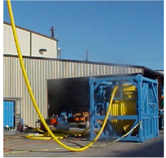
IWOCS reel being tested and spooled in Houston by customer.
