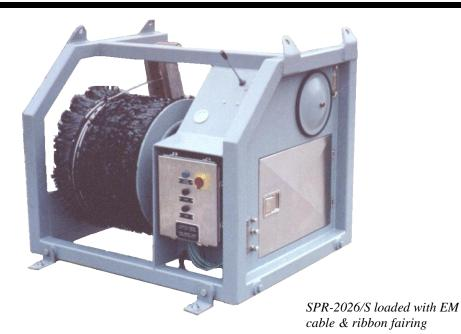
Application: Deployment, recovery and towing of an undulating towfish
